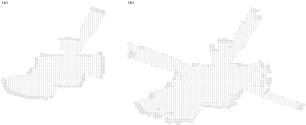
Figure 3. Evidence grids generated from 45 simulated sonar readings for the lower left room in Figure 1 using (a) zero sensor noise and (b) a 0.45 noise setting.
