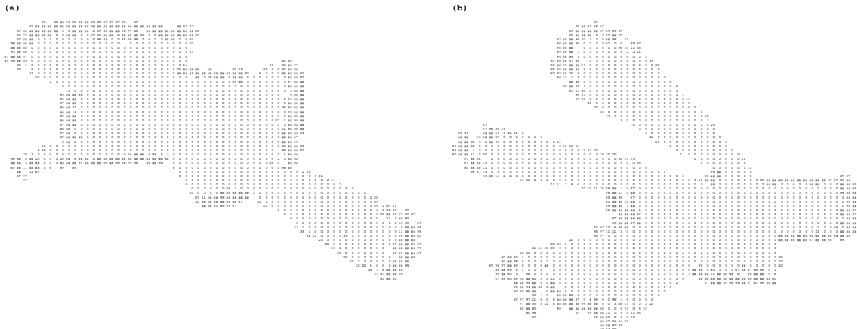
Figure 2. Evidence grids generated from simulated sonar readings for (a) the top left room in Figure 1 and (b) the lower left room in the same figure.
