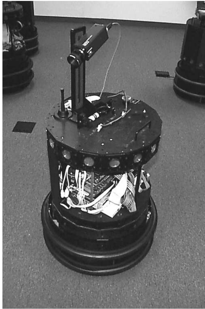
Figure 1. The Nomad 200 mobile robot.
