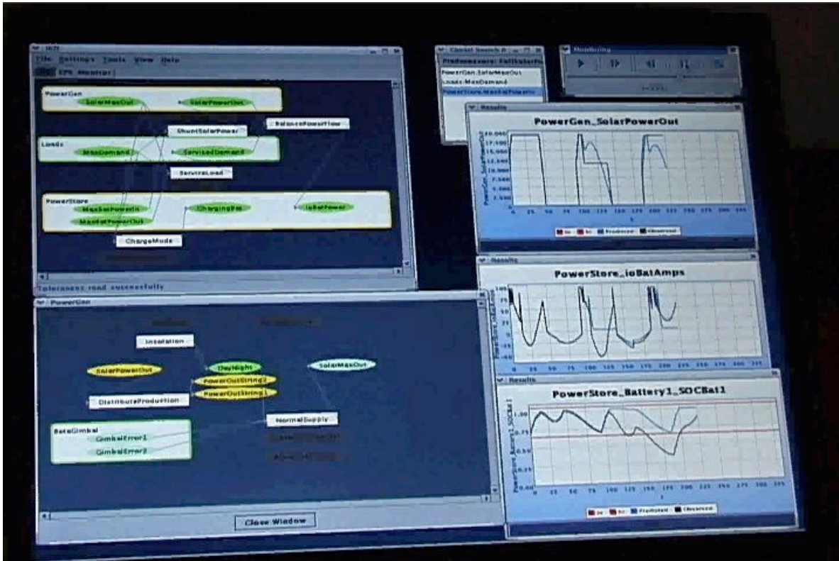
Figure 1: Hierarchical condition layout, with time set to Day 3, when generation is higher than predicted to compensate for under-generation on Day 2. User has 3 variables open and is comparing the timing and nature of the discrepancy between predicted and observed plots.
